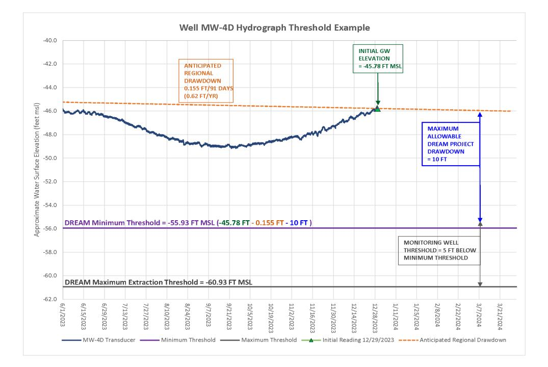
MW-4D is a groundwater monitoring well fitted with a remote monitoring system. Water level data is collected hourly by the remote system and additional manual water level measurements are collected for quality control.
